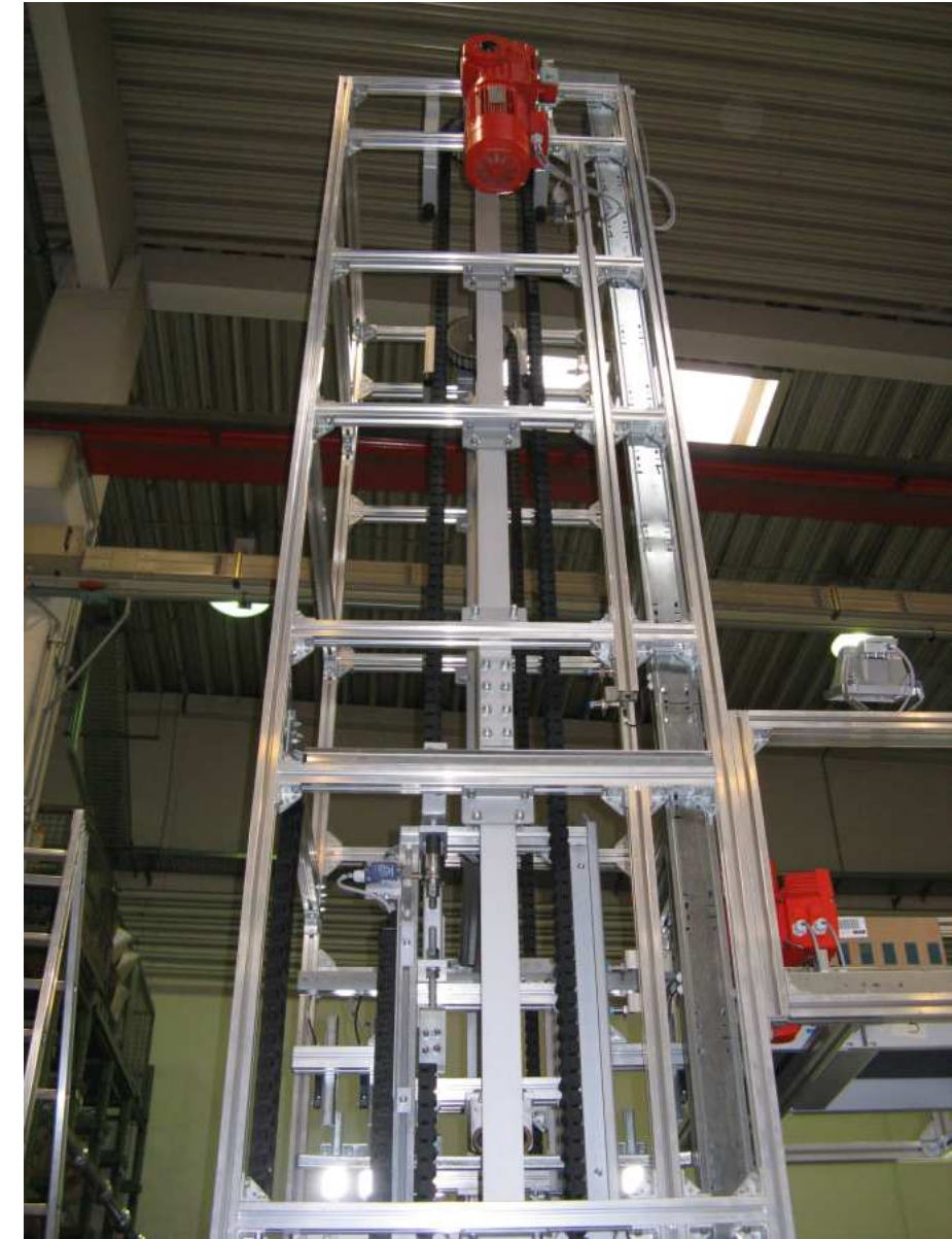
Type: PH253/33/50-All For individual loads up to 200 kg
