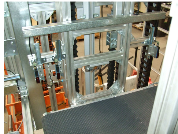
Console with belt conveyor
