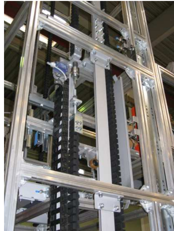
Energy chain, guide profiles, lifting carriage and chain damage monitoring
