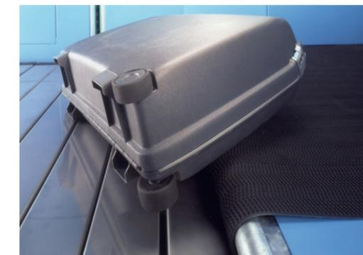
Feed station with internal guides and flat panel platform
